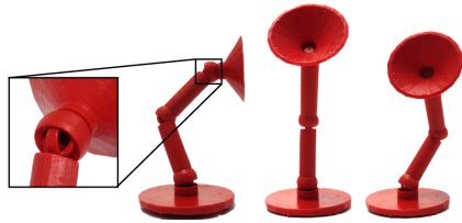
Figure 20: Lamp model printed using joint model from [CCA*12].
